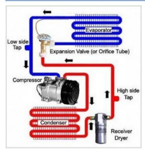
COMPRESSOR: Pumps out refrigerant vapor under high pressure and high heat to the condenser.
